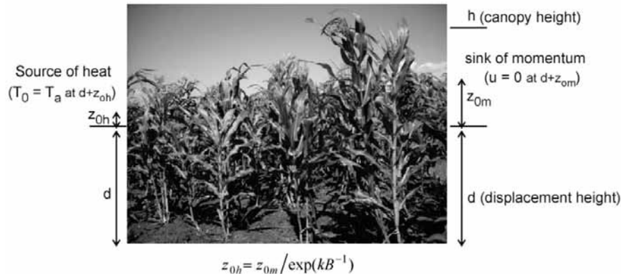
Figure 3.3 An illustration showing the source height of heat ( d+z_{0h} ) and the sink height of momentum ( d+z_{0m} ) and their relation to displacement height ( d ) and the roughness lengths of heat ( z_{0h} ) and momentum transfer ( z_{0m} ).
